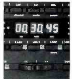
Timer-autolocator control panel
